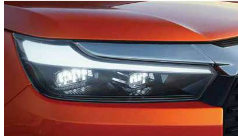
LED Projector Headlamps with Integrated LED DRLs & Turn Indicators
